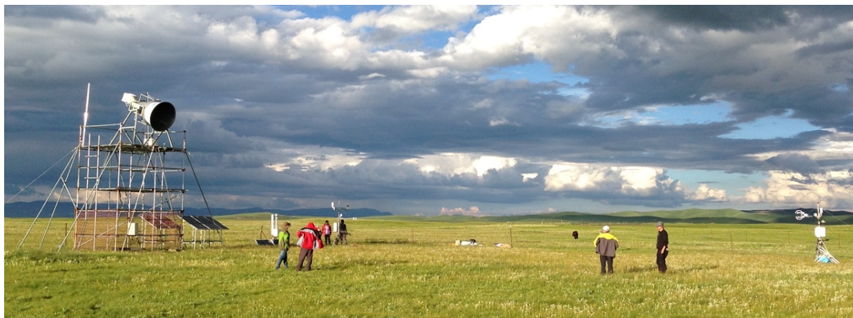
Researchers at the Maqu site of the Tibetan soil moisture and soil temperature observation network (Tibet-Obs), where the European Space Agency has provided an L-band microwave observation system (ELBARA-III) for ground-based observations. GEWEX Quarterly, Vol. 31, No.1, Quarter 1, 2021 pg. 8-10.
